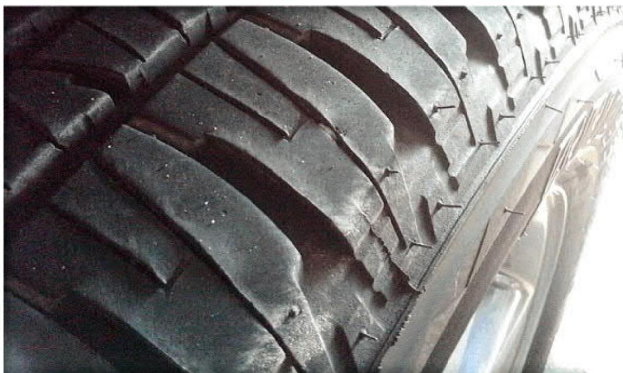
Figure 2: Tyre Shoulder View Example 1 - “NORMAL” Tyre “Feathering” Wear on the Shoulder
